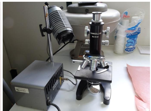
Figure 36: The monocular microscope with an external light source
