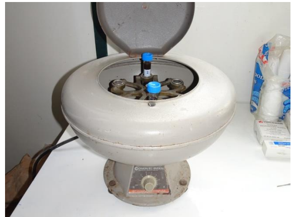
Figure 30: Tubes in the centrifuge
